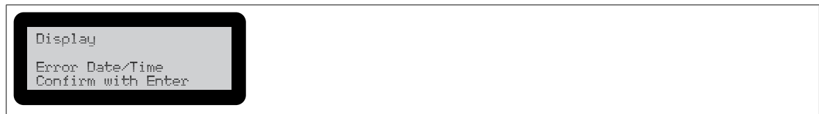
Figure 8.3/1: Error message for exhausted back-up battery
