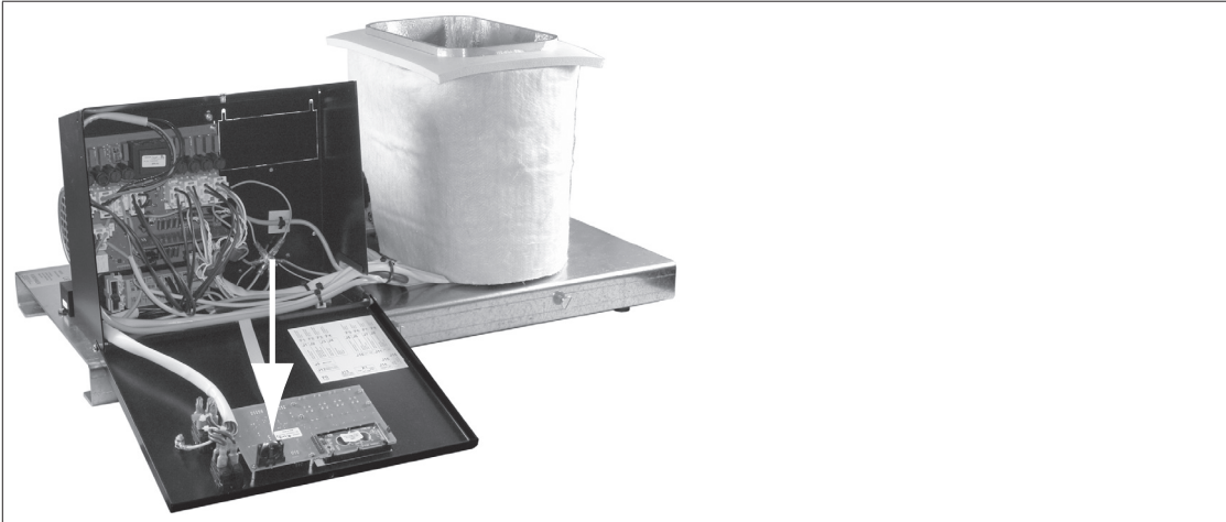
Figure 8.3/3 Position of back-up battery
