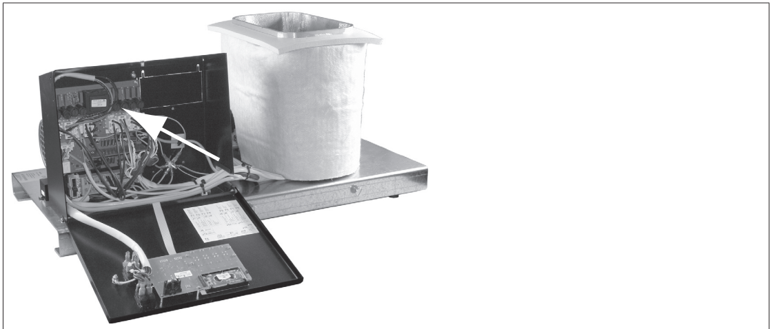
Figure 8.4/1: Position of power section
