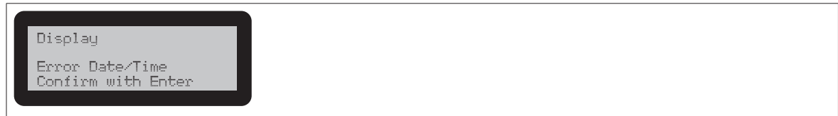
Figure 8.3/1: Error message for exhausted back-up battery
