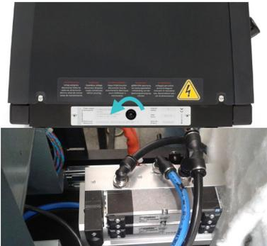
1. Turn off the machine switch on the door of the electrical cabinet next to the pressure regulator. The depressurisation valve releases the pressure from the hydraulic circuit, returning the adhesive to the tank.
