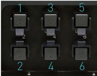
'HB 6000 connect' series melters/applicators are equipped with a hydraulic distributor with a maximum of six outputs. Connect the hoses to the distributor in order, following the numbering in the diagram.
