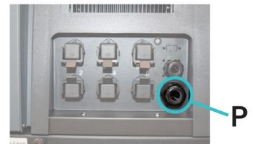
4. Connect the two cable wires to the corresponding terminal/connector. The polarity of the connection must be correct:
