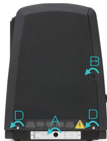
3. To remove the casing from the machine, first you have to separate the electrical cabinet from the tank. To do this, slacken the 1/4 turn screw as indicated (A) and slide it along the guides.
